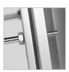
**Gently press the speedring down** towards the softbox, pressing until the back side of the speedring is flush against the metal nuts on the softbox frame poles. You should be able to see the exposed threaded ends of these poles on the outside of the speedring better.
