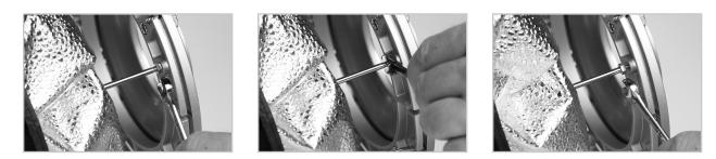
**Loosen the hexagonal metal nuts on the softbox frame poles.** Using the **provided 7mm wrench** (included with each SBA adapter), twist left to loosen the nut on each of the four softbox frame poles.
