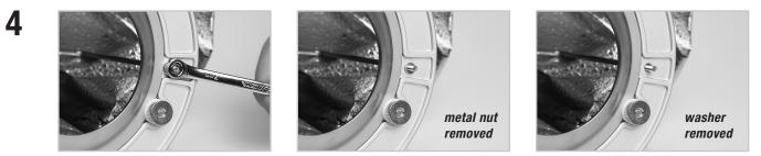
**Loosen and remove these four metal nuts and their washers.** Twist left with the wrench to loosen and remove the metal nuts, then remove the round metal washers located under each nut as well. You will use the removed nuts and washers (4 nuts and 4 washers) again in step 6.
