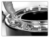
When replacing the flashtubes in your ZEUS RingMaster flash head, first **ensure that the ZEUS power pack is turned OFF and unplugged** from the AC power source. With the power pack turned off, disconnect your flash head(s) from the power pack and allow the units to cool completely.
