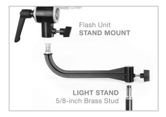
The **Baby Boomer™** is a mounting arm that attaches to the top of your light stand to allow offset mounting and extension of your flash unit 8 inches out from the top of the stand mount. The heavy-duty zinc alloy arm supports all Paul C. Buff™ flash units with a variety of faceplate accessories, attaching to the top coupler of our 13-foot light stands (and similar light stands from other manufacturers having a standard 5/8-inch or smaller mounting stud).
